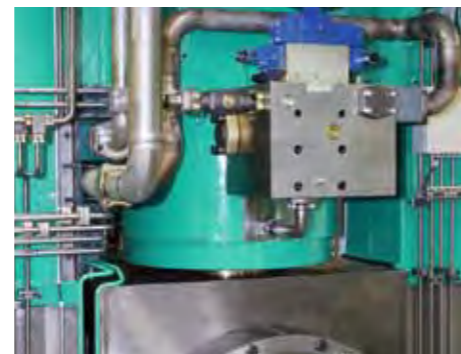
▲ Hydraulic roll force cylinder with direct mounted valve block for high dynamic control characteristic
