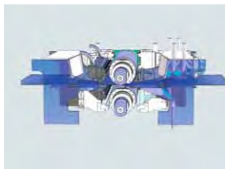
▲ Combined multizone cooling and strip blow-off system
