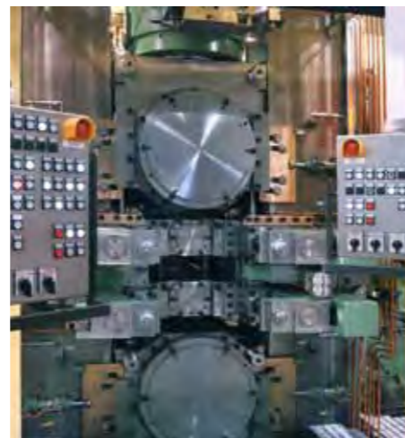
▲ Quarto/S6-high combination rolling mill for mixed product range with low and high carbon steel
