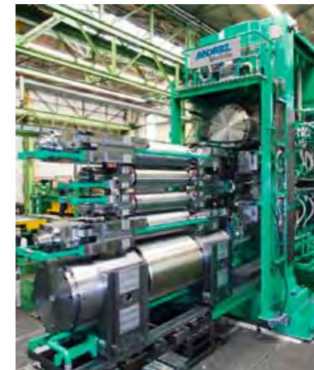
▲ 6-high mill at pre-assembly
