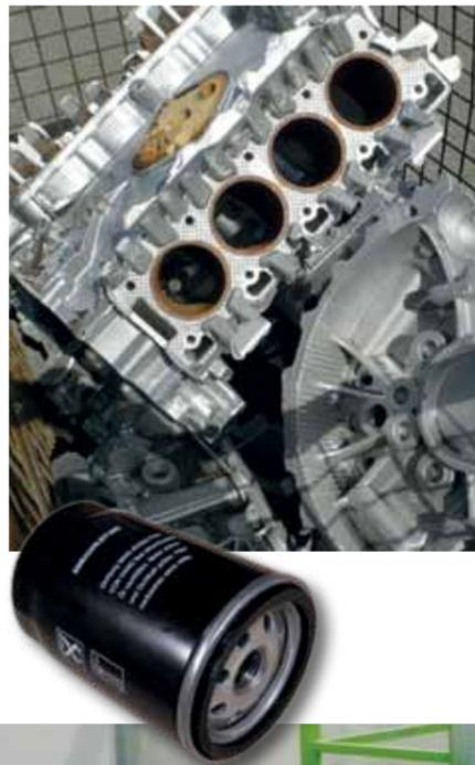
Replaced oil filters from cars and trucks are classified as special waste worldwide. However, they consist of some 60% metals (mainly iron). The oil makes up around 20% of the material mixture. The actual paper filter, rubber sleeves, and other plastic parts make up the remainder.
