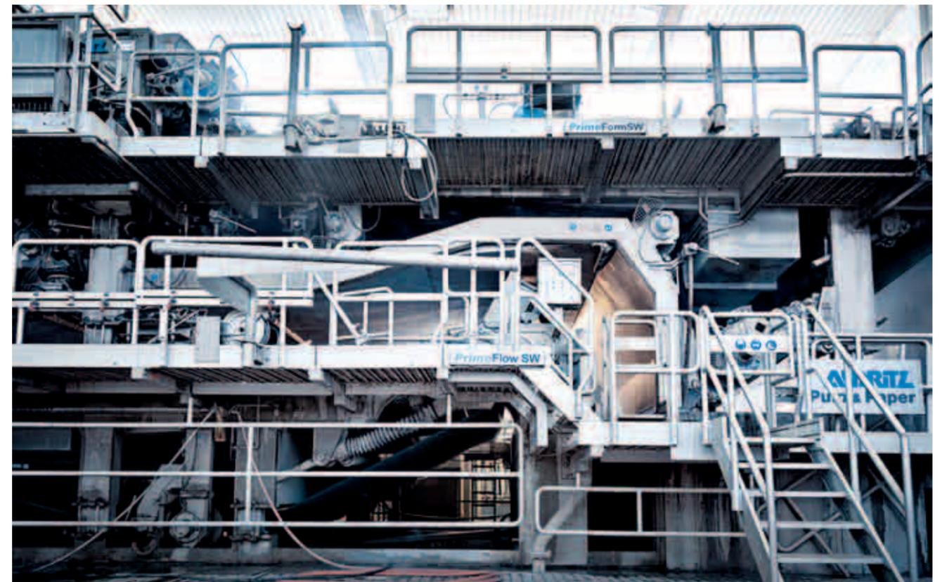
▲ ANDRITZ succeeded in executing the wet end rebuild in only 26 days. The existing cylinder mold formers on PM3 were replaced with a three-layer fourdrinier (*PrimeForm SW*) which included three new *PrimeFlow SW* headboxes. The *PrimeForm HB* is utilized for filler layer dewatering. The existing press section was upgraded with a pick-up roll to allow a closed web run to the press section.
