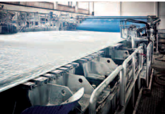
▲ The task was to completely rebuild the wet end on Količevo's PM3 – including a new design hybrid former so it could produce a premium grade of board – in only 10 months from design to start-up.
