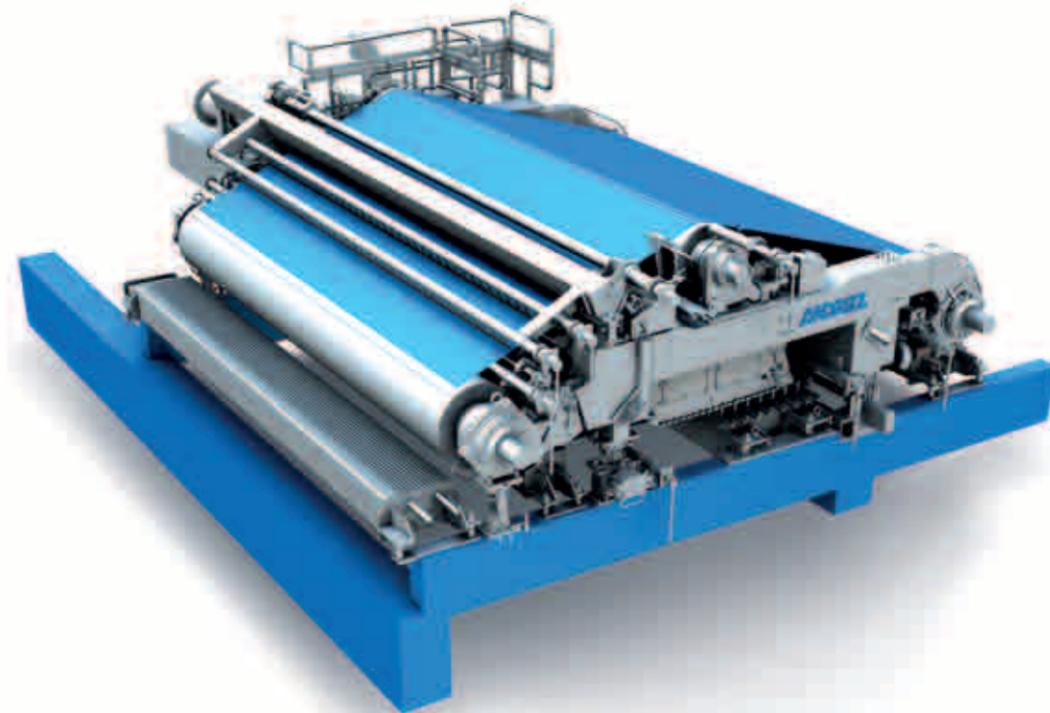
PM3, the machine to be rebuilt, was installed in 1979 by ANDRITZ. It has a trim width of 4.5 m and had eight vacuum formers for grades ranging from 210 up to 500 g/m<sup>2</sup>. Before the rebuild it was producing testliner – a useful commodity grade with small growth potential.
