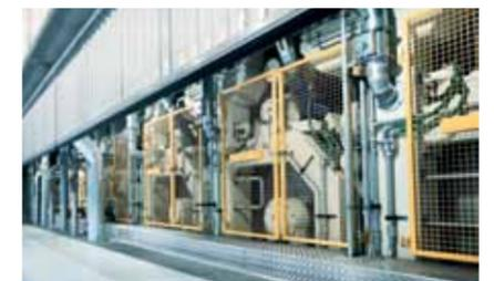
▲ View of the pre-dryer section with vacuum rolls and web stabilizers.
