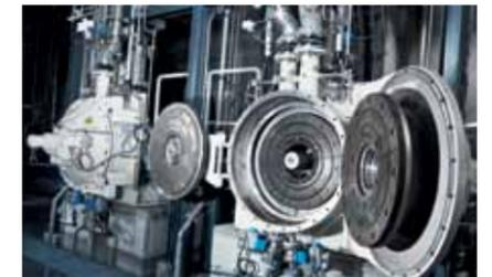
▲ TwinFlo refiners for optimum fiber development in the stock preparation process.
