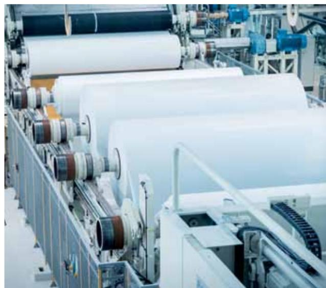
▲ The jumbo reel is rewound and converted to rolls on a two-drum *PrimeWinder* Arcus Evo.
